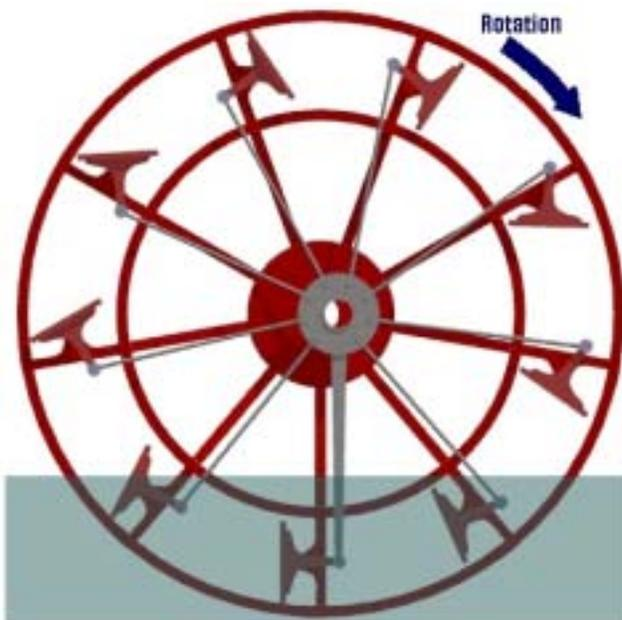
shaped into a lobe and connected to long connecting rods with ball joint ends, which in turn, connected to the paddles. As each paddle struck the water, it was rotated into a perpendicular angle to the water, while the paddle on the top rotation of the wheel, was angled somewhat out of position. The system was most effective, but was troublesome and often broke down.
